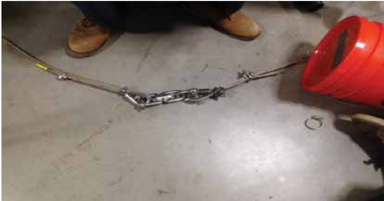
Figure 7 - Example of the junction between buckets and main line using a swivel shackle
