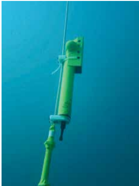
Figure 8 - Example of sensor attached to a short buoy line
